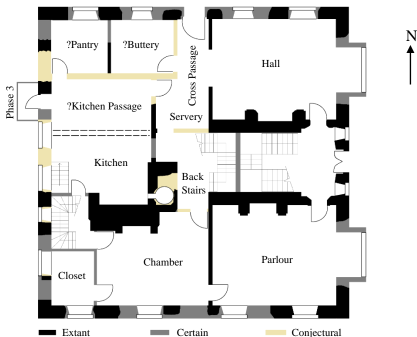
Fig. 8: The Ground Floor Plan of the Main Residential Block in Phase 2 (and 3) (After CMP Fig. 11)
